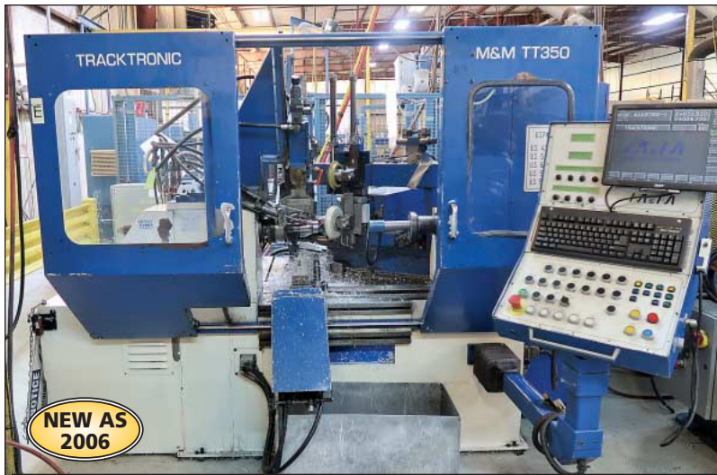
(5) 25.59" x 27.55" M&M Model TT 350 Tracktronic CNC Metal Spinning Machines
